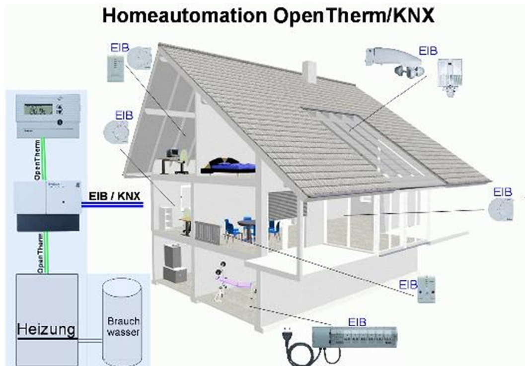
Fig. 3.2.5.8: KNX and OpenTherm (54)
