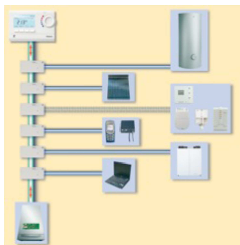
Fig. 3.2.5.5: Multi-point to point OpenTherm communication (52)
